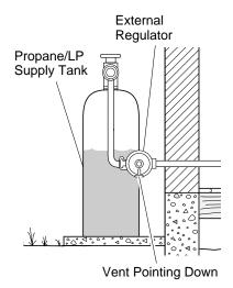
Figure 20 - External Regulator with Vent Pointing Down
